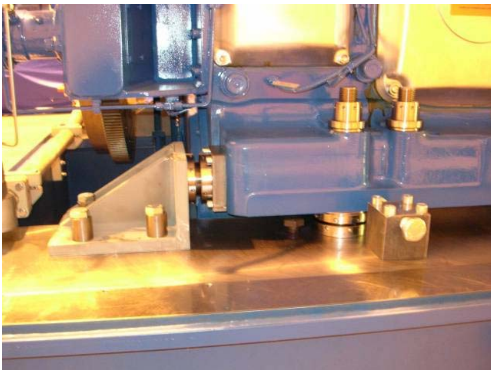
Figure 5.1.6.3 Detail of bracket with Vibracon ® to create a fixed point (alternative for fitted bolts).
