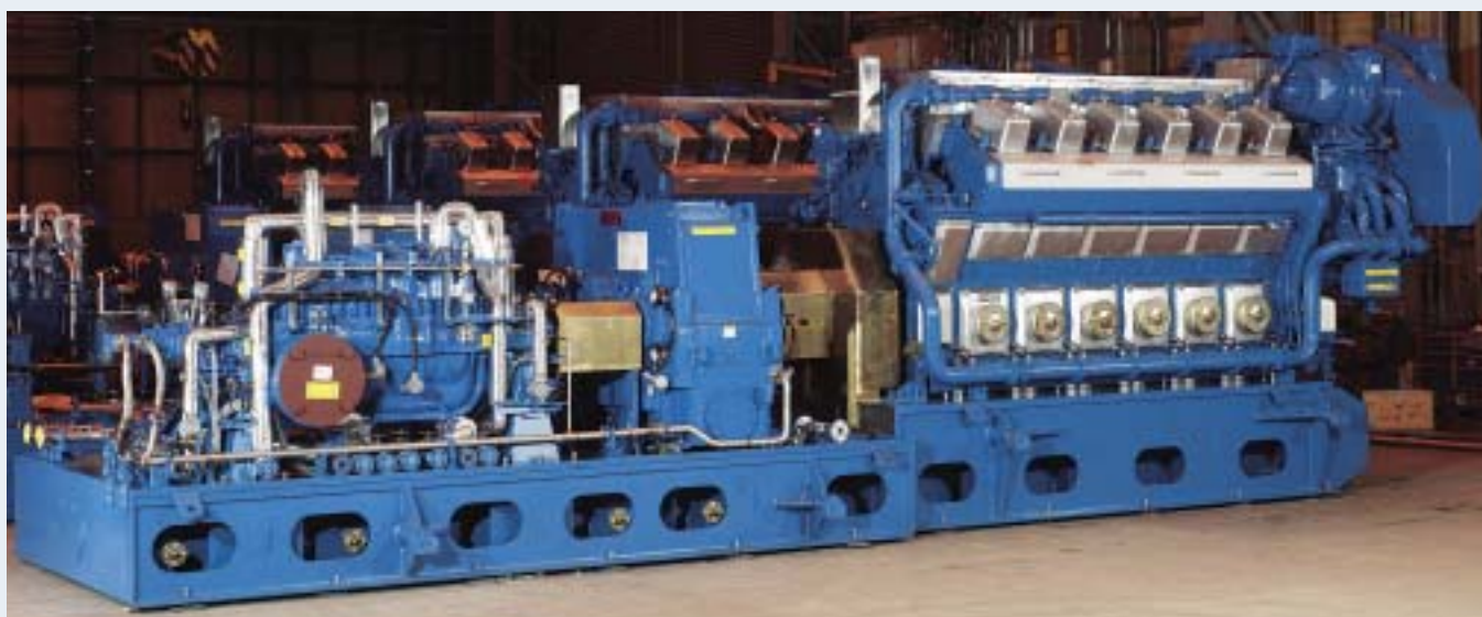
Wärtsilä-Sulzer-Lufkin pumping unit mounted on Vibracon® SM elements, providing easy re-alignment anywhere in the world.
